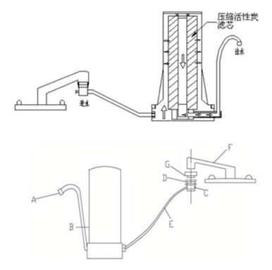
A. spout; B. housing; C. button; D. diverter valve; E. hose; F. faucet; G. adapter
